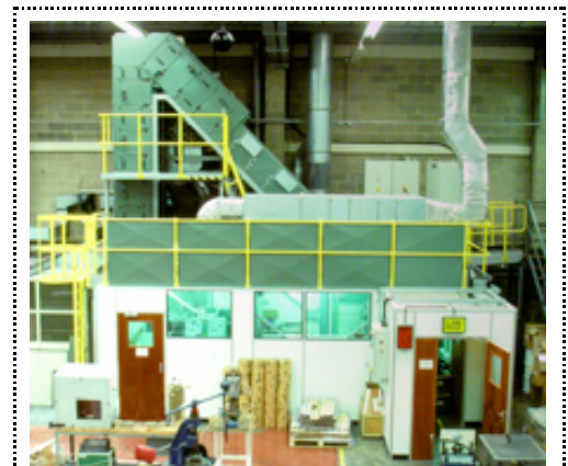
Precision Coating machine in Clean Room (one of the new processes developed)
